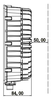
Insure that there is a 50mm gap above the charger to allow for proper ventilation.
