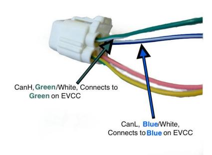
**Note Above:** The Yellow and Pink wires are not used, Refer to the EVCC Manual for more details on EVCC wiring.
