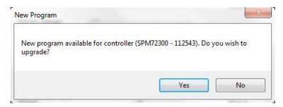
Note: Upgrading the firmware does not change controller configuration. All user settings remain unchanged.
