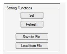
These buttons control the reading and writing of the settings to the controller as well as loading and saving configurations.
