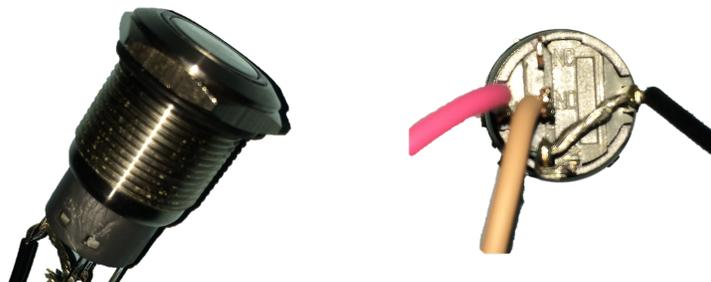
**Figure 6 - Charge Start and ExtInd Wiring**
