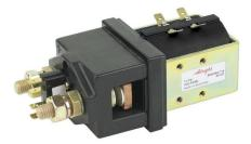
Pictured is a Curtis SW-200 Contractor. Contactors should have a continuous rating of at least 200 amps, with a surge capacity of about 1000 for this controller. Magnetic blowouts are required.
