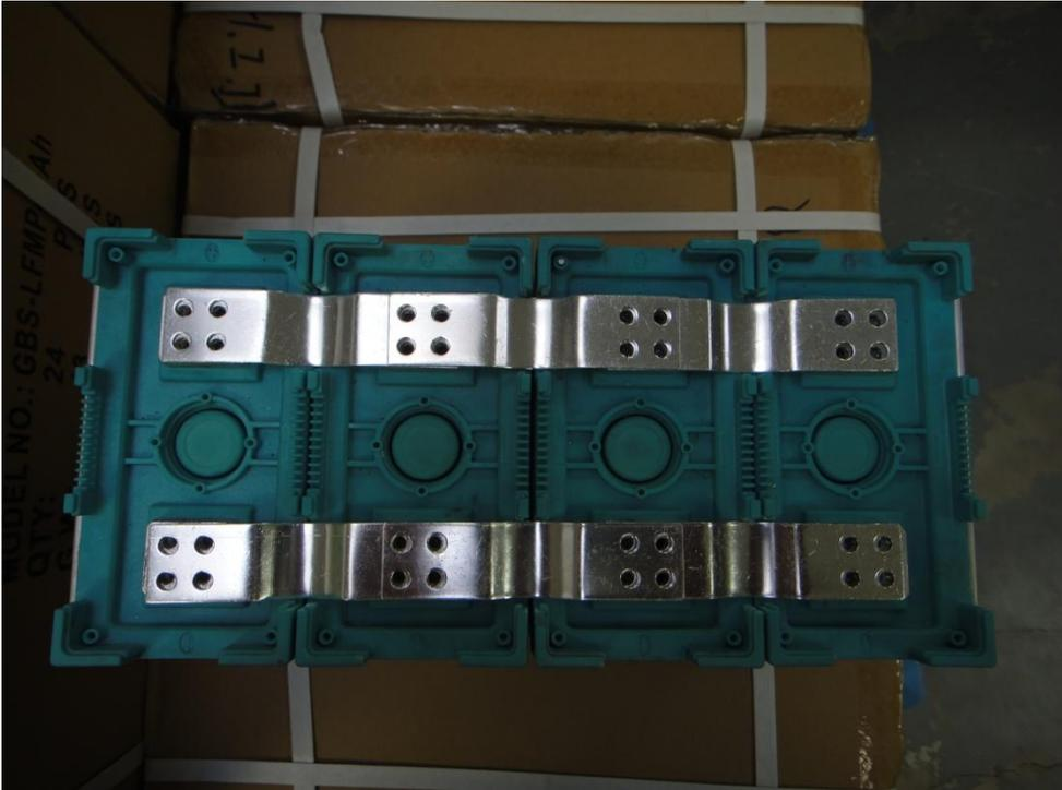
Install jumpers as needed. A thin layer of an electrical conductive grease such as Noalox or similar should be applied to the terminals before installing the jumper. It should also be applied between each jumper if they are stacked more than one high. This helps increase electrical conductivity and ensures long term durability of the connections.
