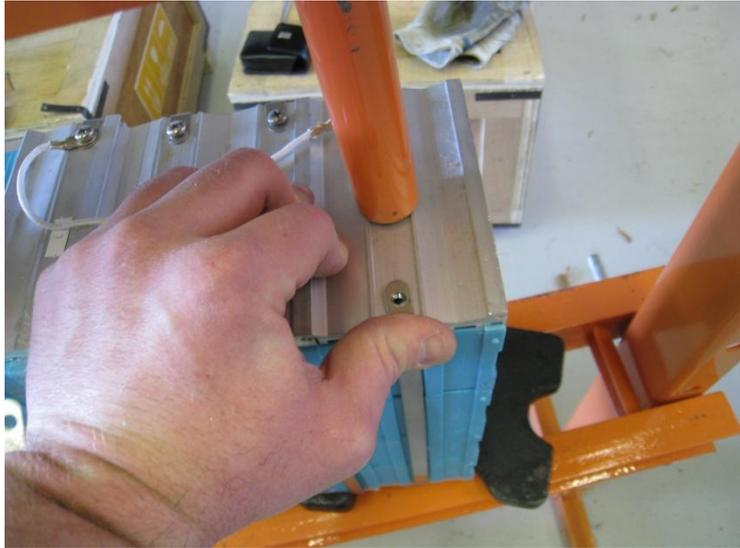
Apply only enough pressure to get the band back over the plate. The closer the press is to the screw the less pressure will be required.
