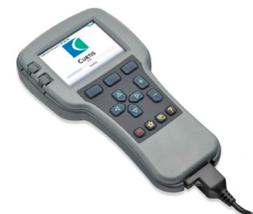
The Curtis Model 1313 Handheld Programmer is ideal for setting parameters and performing diagnostic functions.
